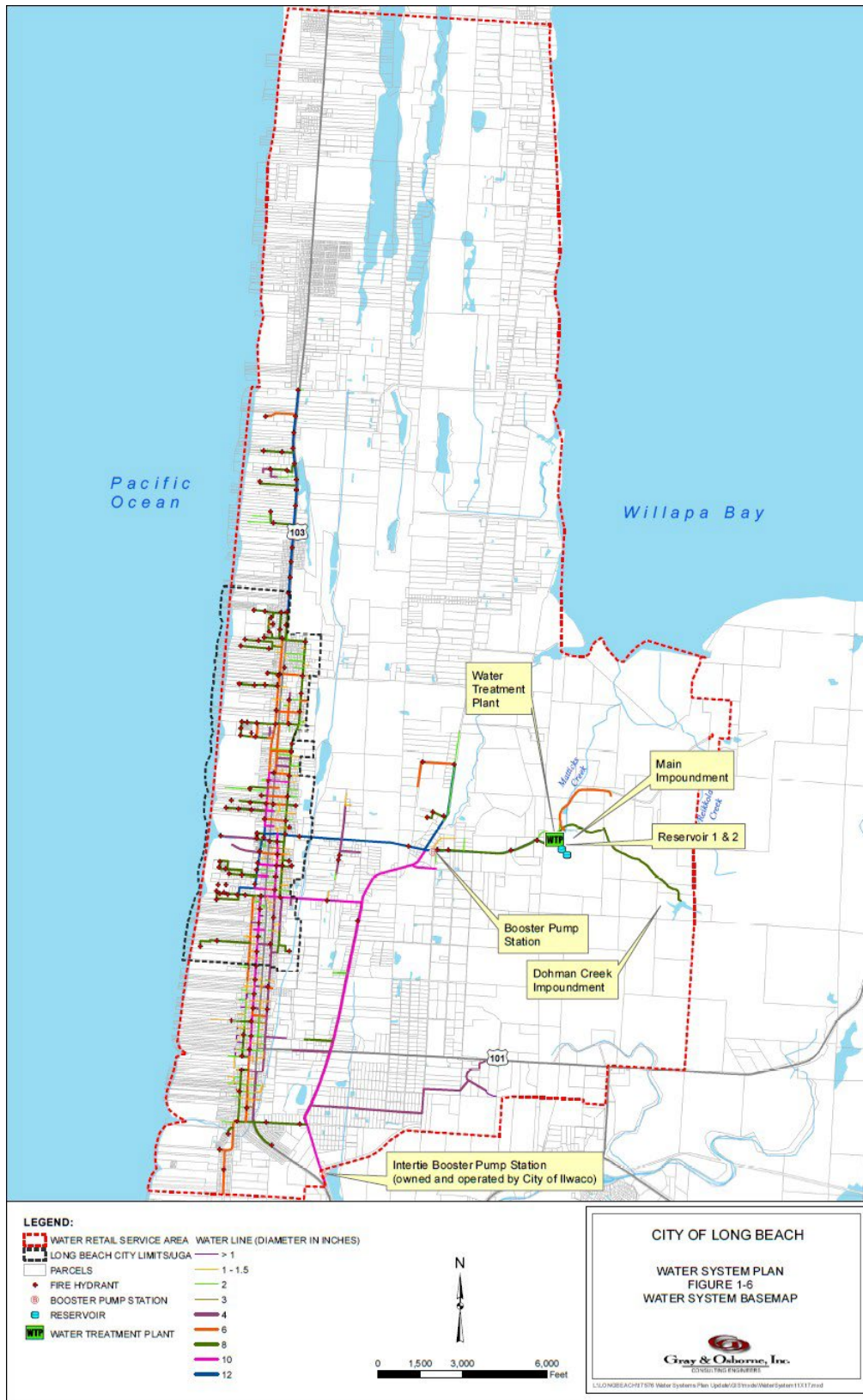
Figure 15: Water system facilities
